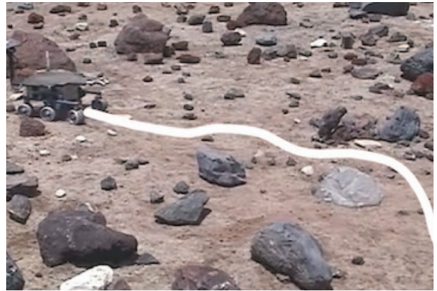
Figure 12. The FIDO rover navigated autonomously among previously unknown obstacles using the graduated density lattice planner. The approximate path the rover followed is shown in white.
