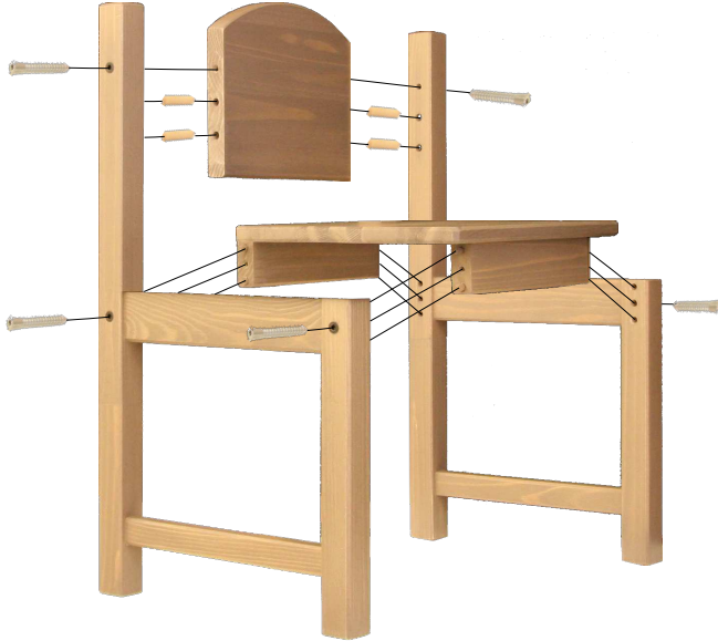
Fig. 3: An exploded view of the complete disassembly of the Sundvik chair. The AND/OR graph and two alternative assembly plans for this chair are shown in Fig. 2
