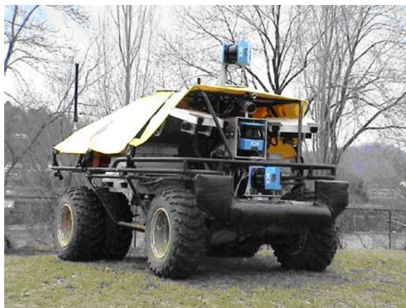
Figure 26: PerceptOR robot. A preliminary version of this algorithm was verified on PerceptOR vehicles, designed to navigate in natural environments.
