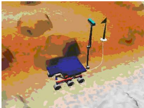
Figure 27: ROAMS simulation of the planner in action. A CLARATy implementation of the state lattice planner is controlling the ROAMS simulation of the Rocky8 rover in this screenshot. The planner generated a smooth path to go around the large rock next to rover in order to drive the rover to explore a crevasse between the two rocks at the left edge of figure.
