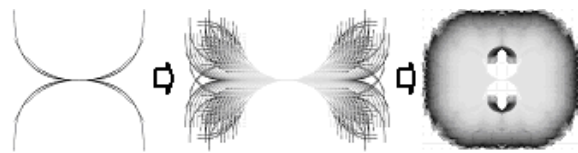
Figure 9: Populating the HLUT Using Dijkstra's Algorithm. Expansion of the lowest cost unexpanded state in the tree is an efficient way of finding the shortest distance to many states at once.
