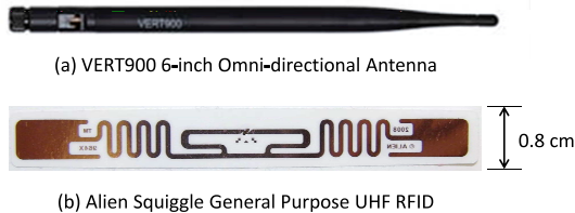
Figure 9—Antenna and commercial UHF RFID used in experiments: (a) We move the VERT900 6-inch vertical antenna in a straight line to emulate a linear antenna array. (b) the Alien Squigggle General Purpose UHF RFID Tags. The sizes of (a) and (b) are not proportional to the real sizes of the devices.
