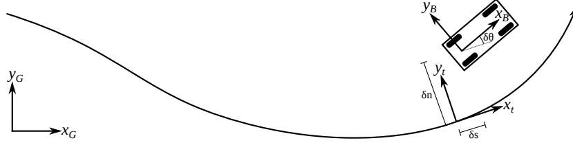
Figure 6.2: The three types of path-following error are cross-track error ( \delta n ), along-track error ( \delta s ), and heading error ( \delta\theta ). The three errors are interrelated since attempts to control one variable often affect the others.
